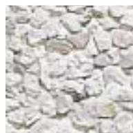
White concrete with aggregates of crushed white marble.
