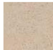
White concrete with aggregates of white anorthosite.
